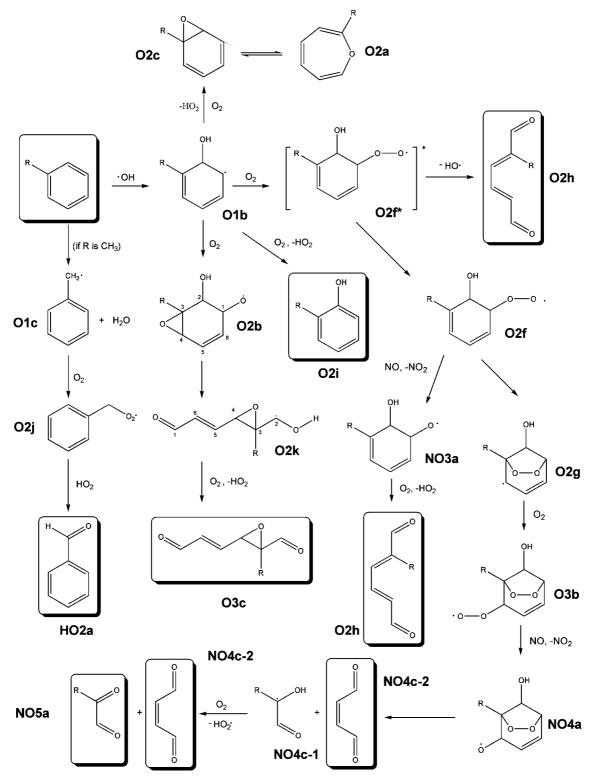
Figure 1. Postulated primary aromatic oxidation mechanism (only ortho OH attack position products are shown).
