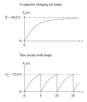
During the rise (that is, for 0 < t < T) the voltage across the capacitor is (see LSM, page 456, last equation in caption for figure 10.39)
