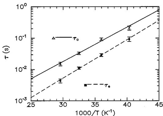
FIG. 2. Arrhenius plot showing the thermally activated behavior of both the mean capture (triangle) and emission (square) times of the RTS for temperatures above 20 K.
