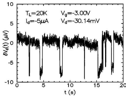
FIG. 1. Time trace of the fluctuation in the drain voltage at a lattice temperature of 20 K. For this pMOS device, a more negative voltage corresponds to a higher-resistance state.
