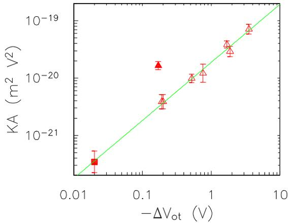
**Figure 1.** Gate-area-scaled noise level (KA) of unirradiated devices versus the threshold shift ( $\Delta V_{ot}$ ) due to net oxide-trapped charge following irradiation of similar devices to a total dose of 100 krad(SiO<sub>2</sub>). The line represents a least-squares fit to all but one of the points.
