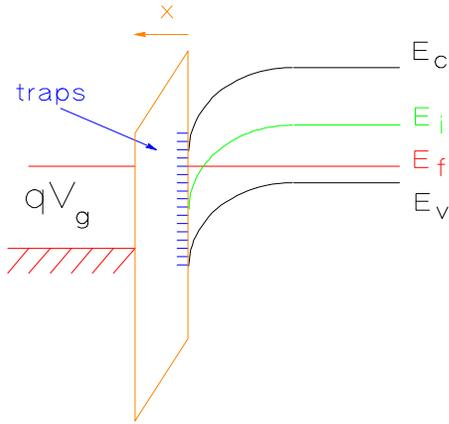
**Figure 3.** Energy band diagram near the Si/SiO<sub>2</sub> interface of an n-channel MOSFET biased in inversion.
