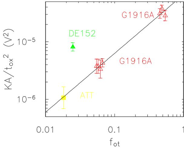
**Figure 4.** Correlation between preirradiation  $1/f$  noise level and oxide-trapping efficiency with the effects associated with variation in oxide-thickness removed.
