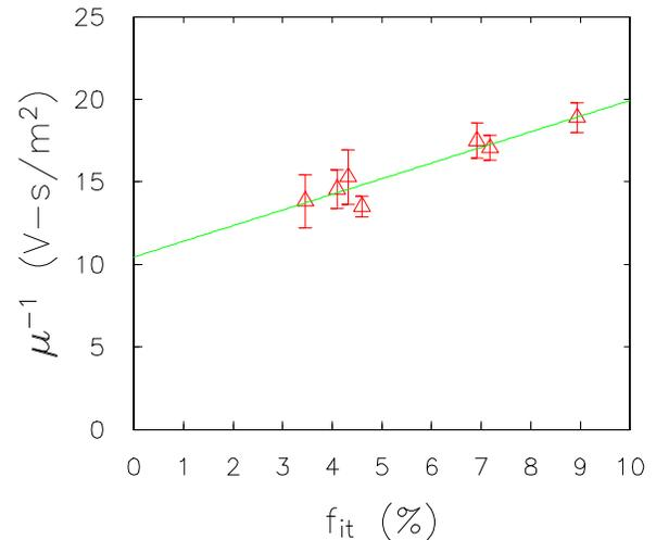
**Figure 6.** Preirradiation inverse channel mobility ( $\mu^{-1}$ ) versus interface-trapping efficiency ( $f_{it}$ ). Values of  $f_{it}$  are derived from  $\Delta V_{it}$ .
