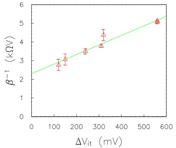
**Figure 5.** Channel resistance parameter  $\beta^{-1}$  of unirradiated devices versus the threshold shift of similar devices due to interface-trapped charge following irradiation to a total dose of 100 krad(SiO<sub>2</sub>).
