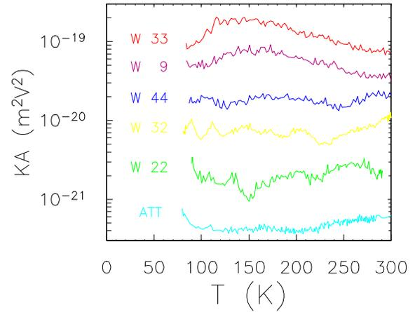
**Figure 2.** Gate-area-scaled noise level KA of selected unirradiated devices versus temperature.
