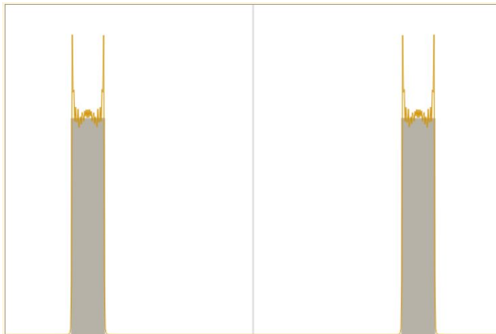
Figure 2: The display of InterferenceSimulator in a short-wavelength situation, demonstrating the classical limit of quantum mechanics (or the geometrical-optics limit of wave optics). The gray boxes show the “ray-optics spotlights” that would be produced if particles behaved classically.
