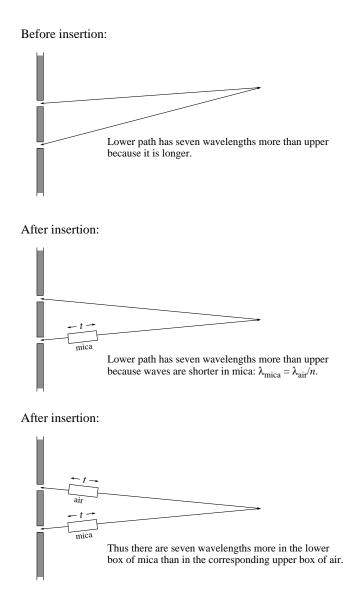
number of wavelengths in air of thickness t is
