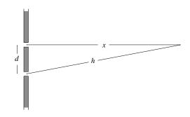
Suppose  $x \gg d$ . Then  $x \approx h$ , so both paths x and h hold the same number of wavelengths, and there is complete constructive interference.
