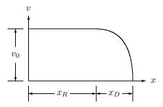
Why do these graphs show  $t_R$  equal to  $t_D$  but  $x_R$  greater than  $x_D$ ? Because the car is going faster during the reaction phase than during the deceleration phase, so if the times were equal then the reaction phase distance would be greater.
