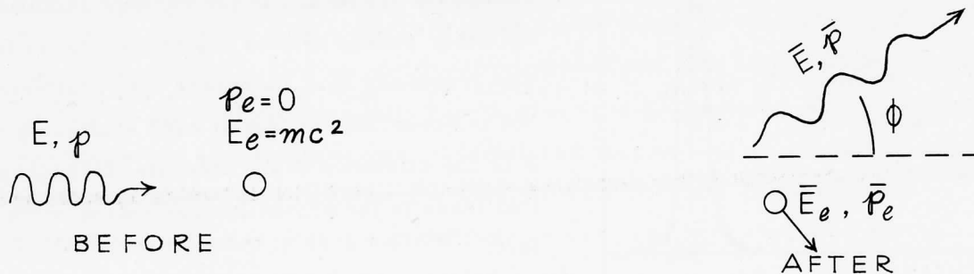
Figure 7. Symbols for analysis of Compton scattering of a photon
